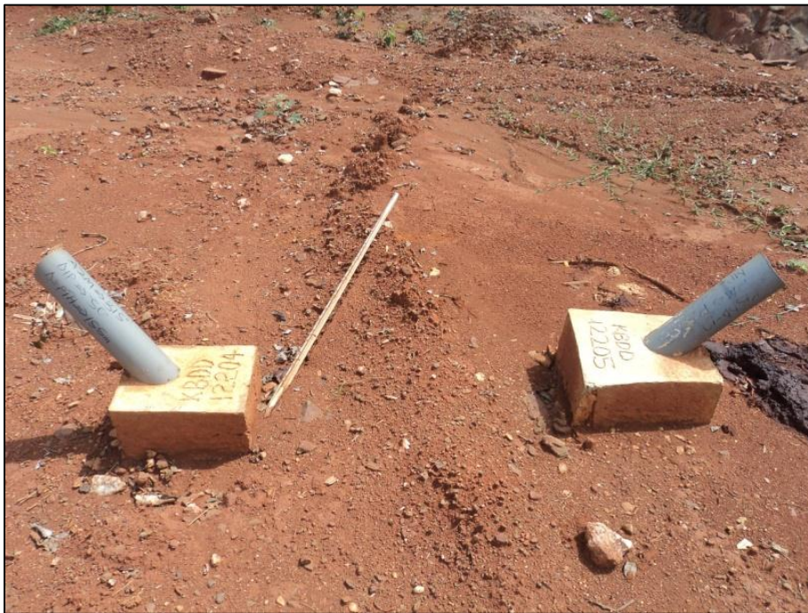
Figure 27 After drilling the collars have been capped and labelled.
