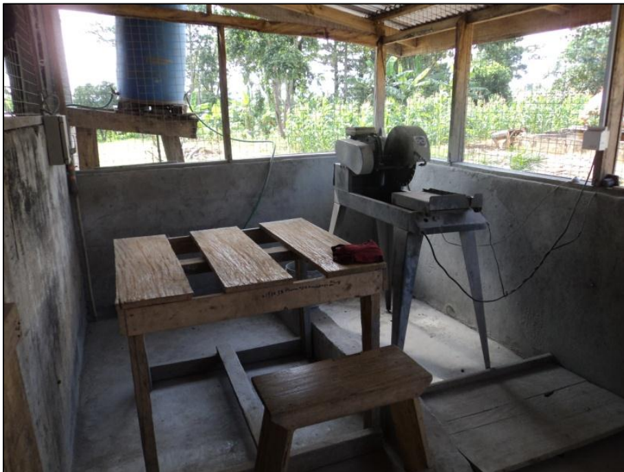
Figure 31 Core saw for sawing core in half longitudinally ready for sampling.
